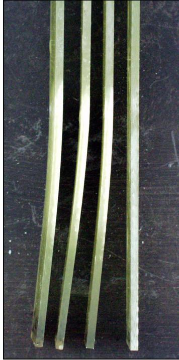
Figure 6: Permanent deformation of  $[\#45^\circ]_8$  specimens after removing the lower clamp.
