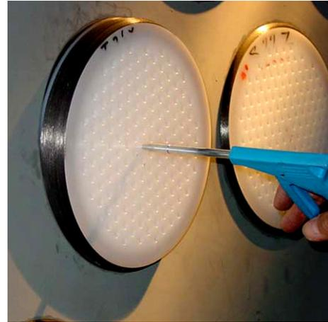
Fig. 3. Positioning of the composite disc in the pedestals of the ball-joint (courtesy of Rijkswaterstaat).
