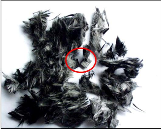
Fig. 11. Undigested epoxy matrix parts after 5 h digestion time.
