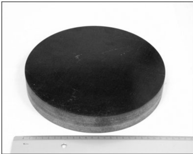
FIG. 3. View of the polyester/polyester disc with Teflon coating.
