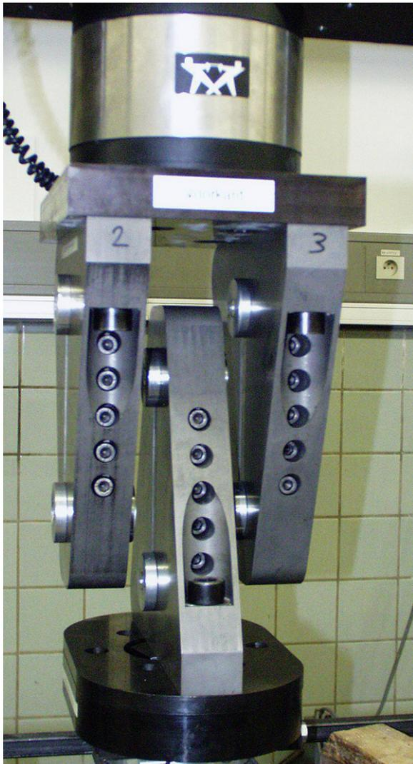
Fig. 8. The final design, mounted on the tensile machine.
