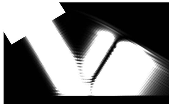
FIG. 6. Schoch effect: formation of specular lobes by an incident 4 MHz ultrasonic Gaussian beam on an aluminum plate under the Rayleigh angle.
