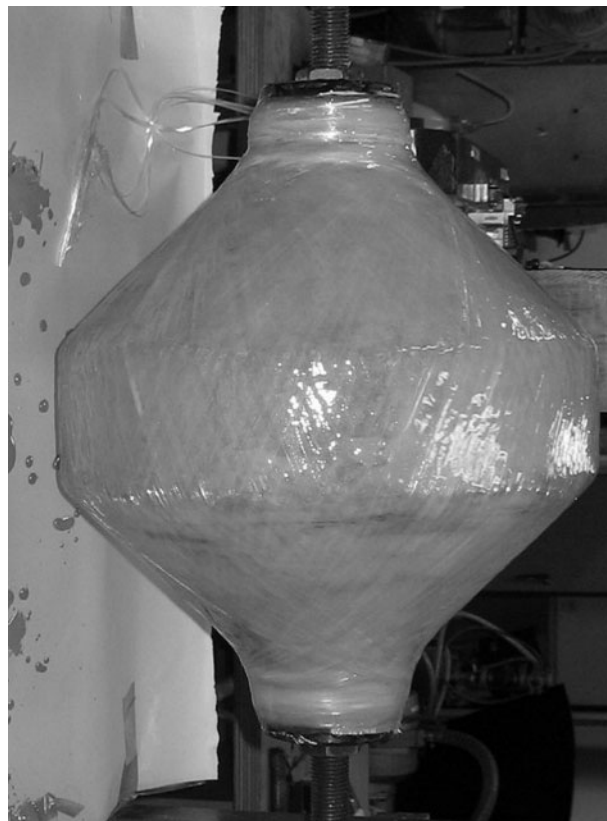
4 Different shapes for point absorbers are considered within SEEWEC; this is possible scaled shape of point absorber which was studied extensively during project; it was made on winding machine in laboratory at Ghent University
