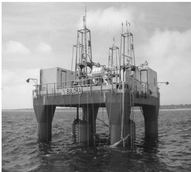
1 One third scale model 'Buldra', used for extensive testing at south coast of Norway since February 2005, whose main objective is development of second generation wave energy converter through extensive use of experience gained from monitoring this scale model
