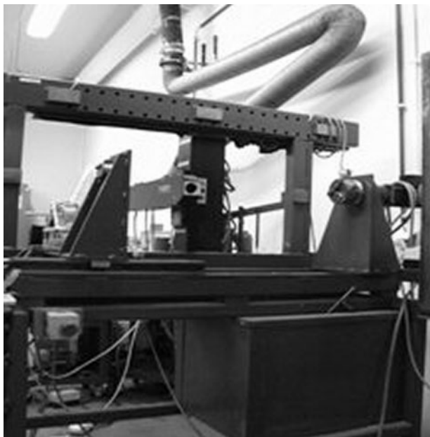
3 Small filament winding machine in laboratory of Ghent University which was used to make laboratory scale test samples discussed further on in this paper
