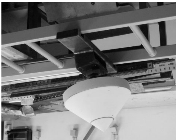
7 Polyurethane cone test sample attached to ladder of slamming set-up: the cone is chosen as reference test case
