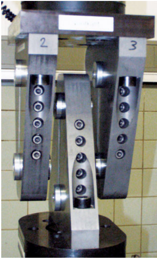
FIG. 8. The modified three-rail shear setup, as presented in [22]. [Color figure can be viewed in the online issue, which is available at www.interscience.wiley.com .]
