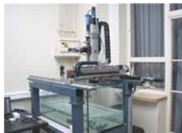
Ultrasound scanning set-up with five degrees of freedom
