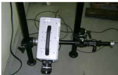
Digital high-speed camera (up to 250 000 frames per second)
