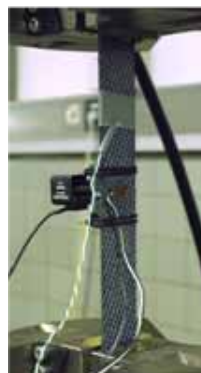
Fatigue testing of thermoplastic composite
