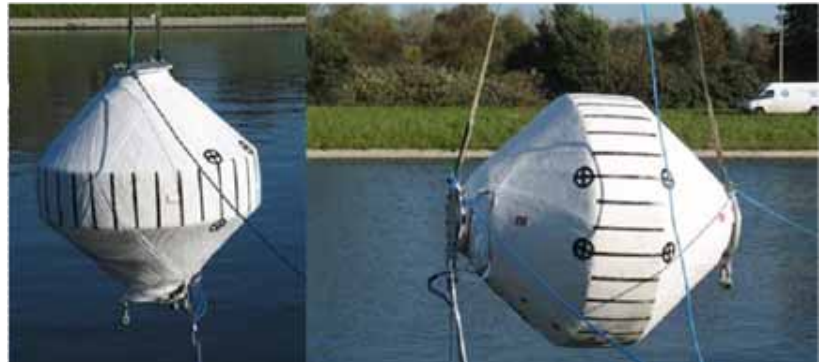
Large-scale slamming tests at the canal in Ghent
