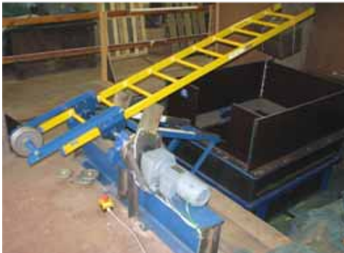
UGent lab-scale slamming set-up for wave impact
