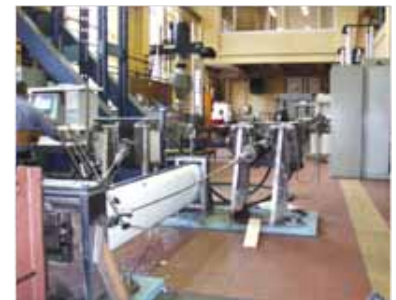
Testing of pre-stressed section of sailing mast
