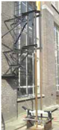
Drop weight test (height 12 m)
