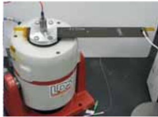
Vibration testing of carbon/epoxy coupons
