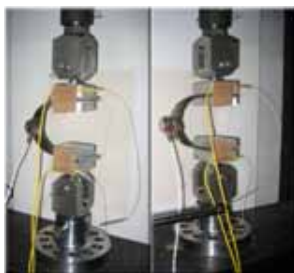
Testing of carbon/epoxy C-profile with embedded optical fibres
