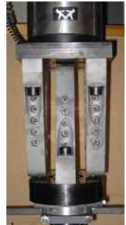
Rail shear fixture for fatigue testing in pure shear
