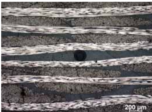
Embedded optical fibre sensors in thermoplastic composite
