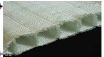
Three-dimensional woven glass fibre preform (TU Dresden)
