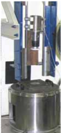
Drop weight test (height 3 m)
