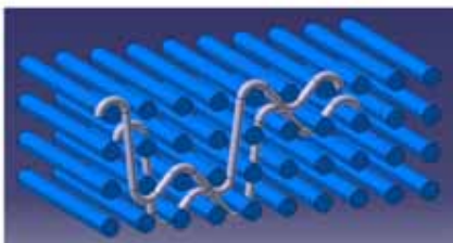
Simulation of three-dimensional yarn in fibrous preform
