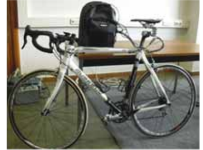
Instrumented racing bicycle for field testing of comfort and vibration levels
