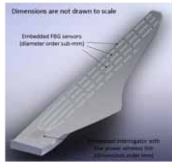
Future turbine blade with embedded smart sensing
