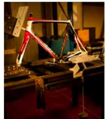
UGent all-in-one test set-up for fatigue testing of racing bicycles
