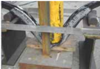
Drop weight testing of bumper component
