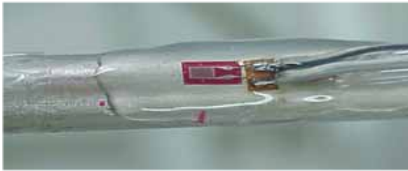
Strain gauge measurement on sailing mast rigging
