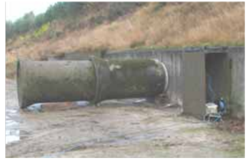
Large-scale blast tests with shock tube at the military domain in Brasschaat
